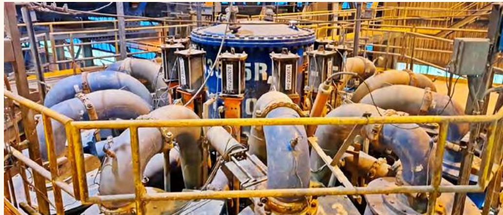
Figure 1. Acoustic sensor in the overflow of each hydrocyclone.
